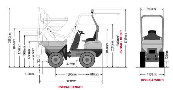
MAX SAFE CARRYING WEIGHT: 1,000KG | LEVELLED CAPACITY: 415L | HEAPED CAPACITY: 525L
