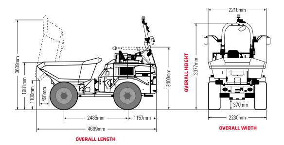
MAX SAFE CARRYING WEIGHT: 6,000KG | LEVELLED CAPACITY: 2,350L | HEAPED CAPACITY: 3,150L
