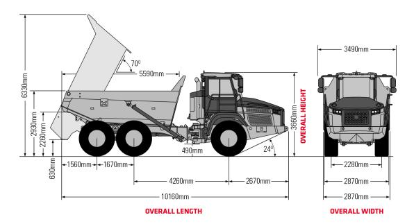
LEVELLED CAPACITY: 13,700L | HEAPED CAPACITY: 18,300L
