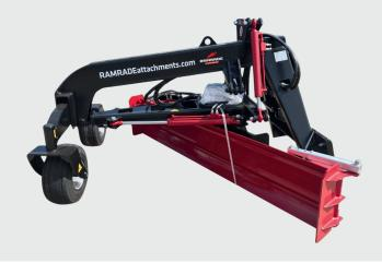
The RAMRADE Cobra Grader Blade, ideal for inaccessible sites, features an Italian-made design with a reversible double-bevel cutting edge for easy replacement. Its hydraulic leveling blade offers 40 cm lateral adjustment, 34° rotation, and compatibility with 2D or 3D GPS systems, ensuring transformative capability for your skid steer.
