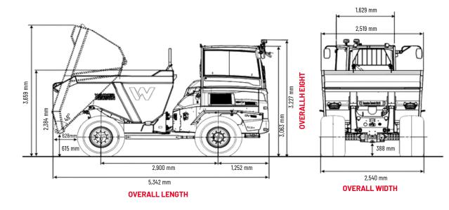
MAX SAFE CARRYING WEIGHT: 12,500KG | LEVELLED CAPACITY: 5900L | HEAPED CAPACITY: 7000L
